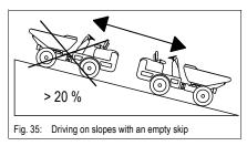
When driving on slopes (> 20 %) with an empty skip, the skip must always face downhill since the heavier part of the machine – in this case the engine – must face uphill to prevent the machine from tipping over.
