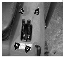
Fig. 44: Dumping in and out 1501S
