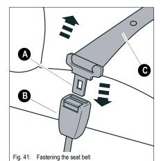
Seat belt **C** is for the driver's safety during work on construction sites and during road travel.
