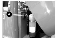
Fig. 42: Oil level indicator on the hydraulic oil tank 1001/
