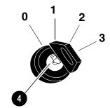
Fig. 26: Preheating start switch
