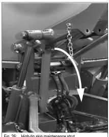
Fig. 26: High-tip skip maintenance strut
