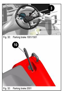
Parking brake with mechanical braking effect on the front axle.
