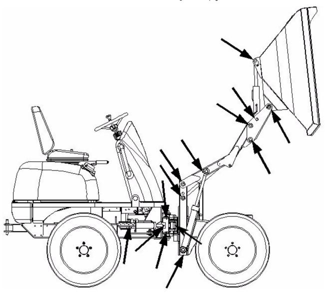
Apply multipurpose lithium grease with an MoS² additive to all lubrication points indicated.
