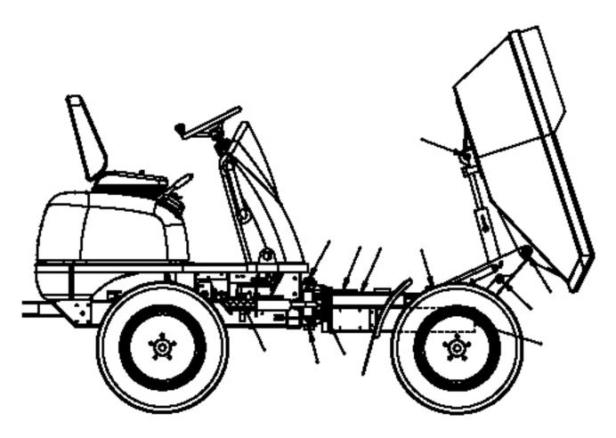
Apply multipurpose lithium grease with an MoS² additive to all lubrication points indicated.
