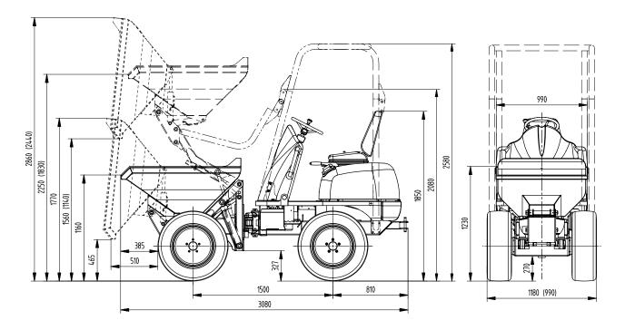
Fig. 53: Machine dimensions (model 1001)
