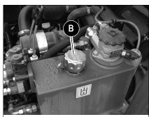
Fig. 43: Hydraulic oil tank
