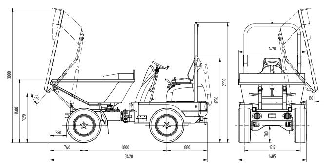
Fig. 58: Machine dimensions (model 2001)
