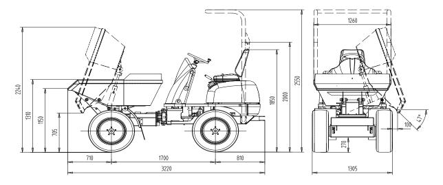
Fig. 55: Machine dimensions (model 1501S)
