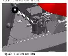
Filler inlet **A** for the fuel tank is located under the engine cover, on the right in driving direction.
