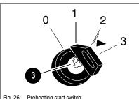
Fig. 26: Preheating start switch
