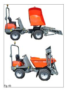
The loader unit has been designed for raising loose material up to 300 kg. The 2001 SLE is not suitable for excavating or pushing heavy material.
