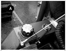
Fig. 30: Fuel filler inlet 1001/1501
