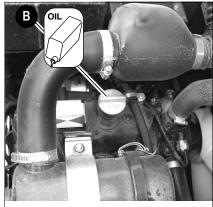
Fig. 35: Filling up engine oil
