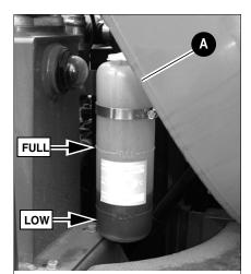
Fig. 36: Expansion tank for coolant
