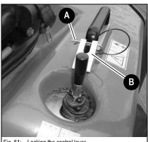
Fig. 51: Locking the control lever
