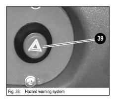
Pressing switch 39 switches the hazard warning system on and off.
