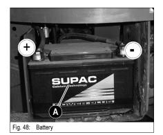
Battery **A** is located underneath the engine cover. The battery is "maintenance-free". However have the battery checked at regular intervals to make sure the electrolyte level is between the MIN and MAX marks.
