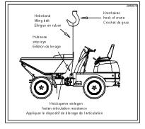
Fig. 23: Loading the dumper
