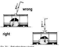
Fig. 31: Refuelling from a barrel
