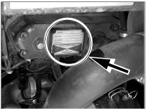
Yanmar diesel engine number
