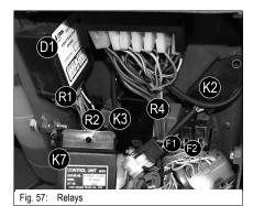
The relays are located in the relay box under the cab, next to the swivelling console
