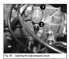
There are two HP pressure limiting valves on the pump under the floor panel, one on the upper left and the other on lower left.
