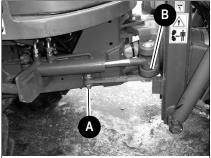
Fig. 50: Centre pivot strut
