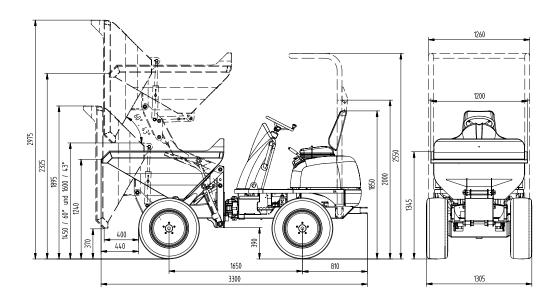
Fig. 54: Machine dimensions (model 1501)
