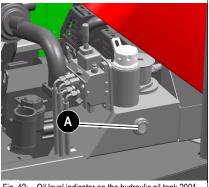
Fig. 42: Oil level indicator on the hydraulic oil tank 2001
