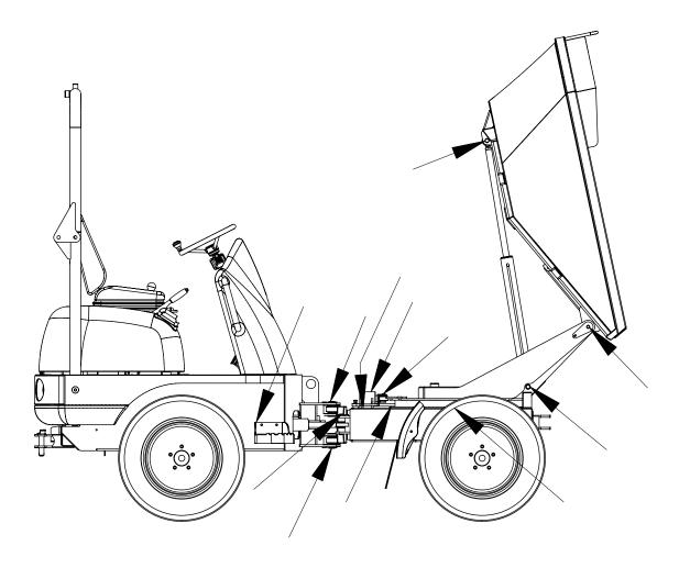
Apply multipurpose lithium grease with an MoS<sup>2</sup> additive to all lubrication points indicated
